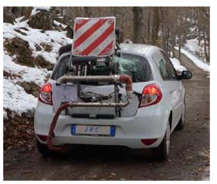
A real-driving test performed by the JRC using PEMS © EU, 2013 Source: http://ec.europa.eu/dgs/jrc/index.cfm?id=1410&dt\_code=NWS&obj\_id=16180&ori=RSS
